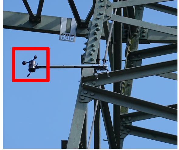
Fig. 1. Fiber-optic anemometer (FOA) on transmission tower
